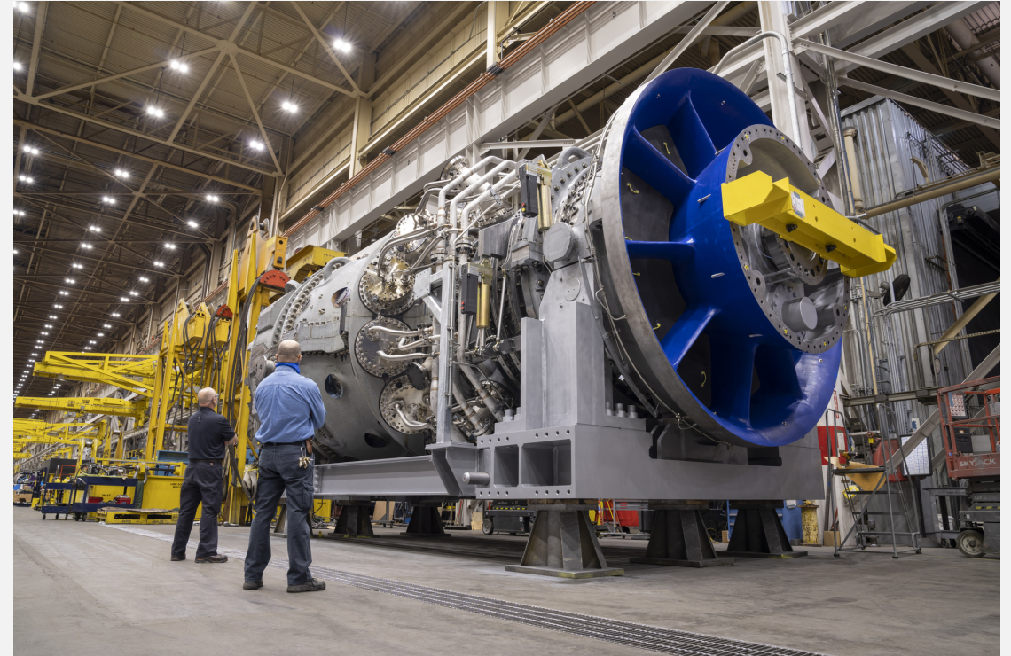
Technicians with a 7HA.03 gas turbine in Greenville, SC
